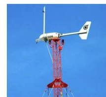
Figure 2. Wind energy generator installed on a 33m height mast at the Energy Laboratory site
