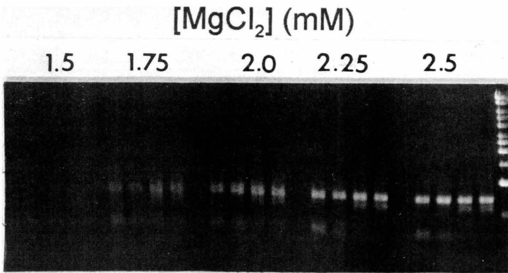
Figure 10. Variation of the RAPD profiles generated by the decamer B4, in response to a gradient of MgCl<sub>2</sub> concentrations. The arrow indicates the position of the RAPD B4<sub>570</sub>.
