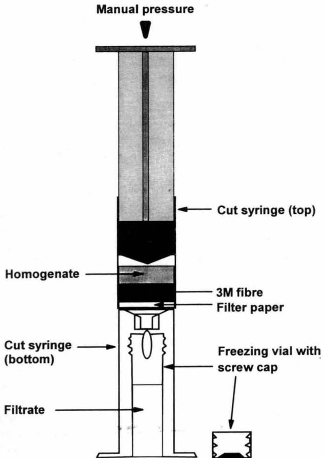
Figure 1. Device used for the rapid filtration of the protein extracts.
