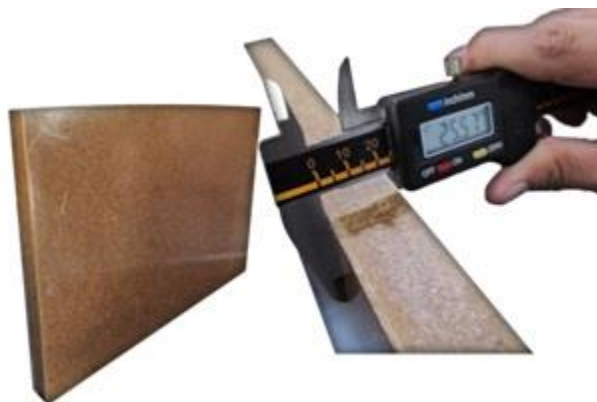
Fig. 3. A WPC board with approximately 25-mm-thick
