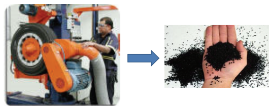
FIGURE 1: Obtaining of flake-like particles from wasted tires.
