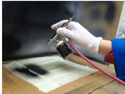
Figure 1. Spray deposition of CNT film onto glass fibers.
