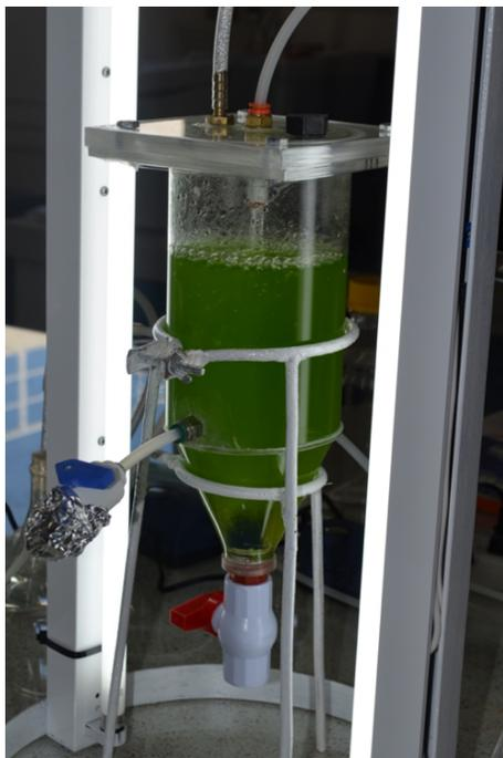
Fig. 1. Conical-cylindrical photobioreactor.
