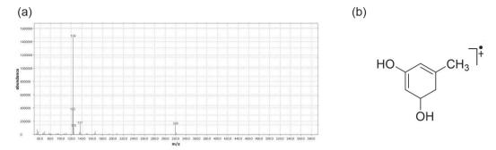
Figure 1. (a) Fragmentation pattern of one of the components ( $t_R$  17.8 min) in fraction B5 showing a molecular ion at *m/z* 320 and a base peak at *m/z* 124; (b) structure corresponding to the base peak fragment at *m/z* 124 ( $C_7H_8O_2$ ).
