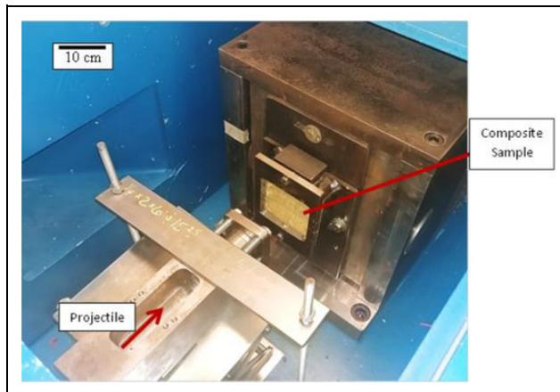
**Figure 3.** High-velocity impact testing area of the nitrogen gas gun. Samples were clamped on a steel bracket. A new sample was used on each impact testing.
