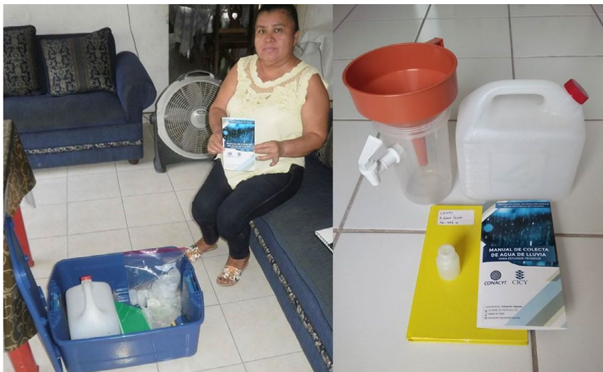
FIGURE 1 Sampling collection kits and manuals for sampling, storage and preservation of the water samples
