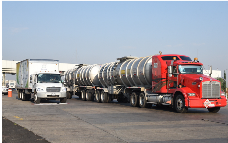
Figure 1.7: Example of a T3-S2-R4 tanker truck
