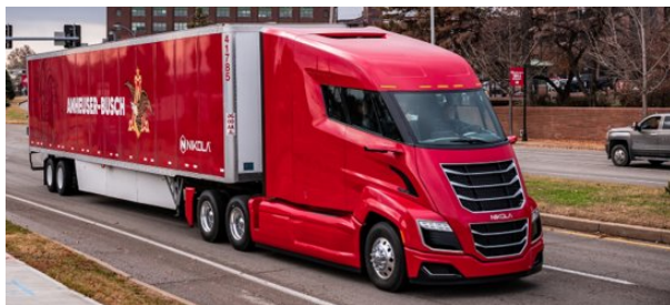
(a) FC Truck: Tractor in a 6x4 configuration, America
