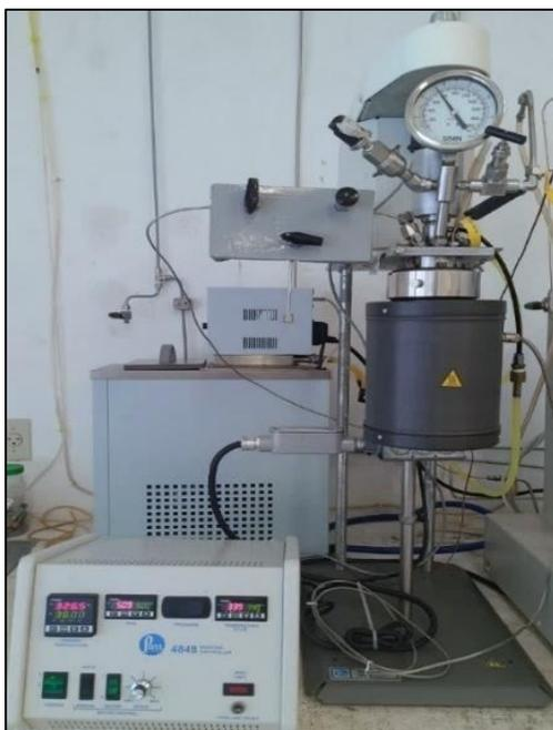
**Figura 2. 25.** Reactor batch marca Parr instrument company modelo 4598
