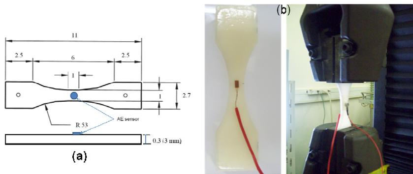
Figure 2.- a) Dog bone shape dimensions, b) longitudinal gauge and attached AE sensor.
