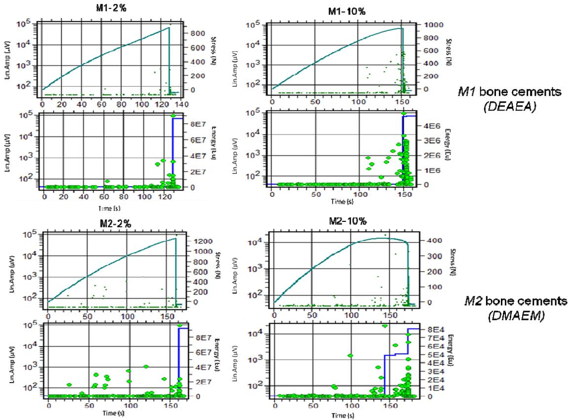
Figure 4.- AE signal analysis for M1 and M2 bone cements.
