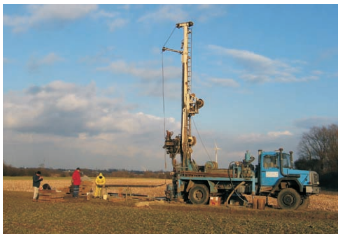
Figure 2. Coring at the Wunstorf drill site in March 2006.
