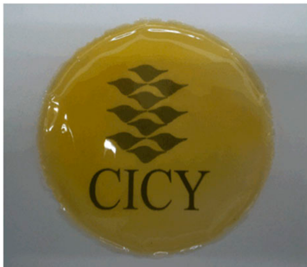
Figure 5. Dense membrane of the polyamide DEAIA-MIMA.
